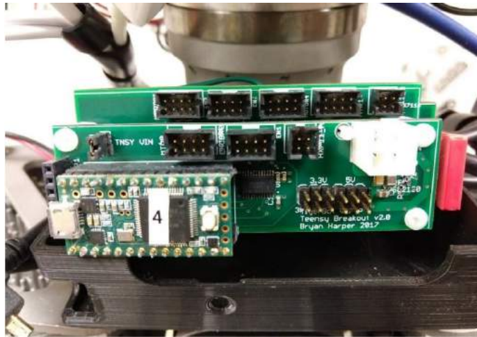
Figure 5.6: Three layered PCB stack to control 3 joints per PCB stack.
