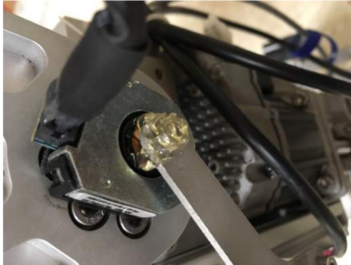
Figure 8.2: Temporary fix for the slippage in the external encoder of the knee joint.
