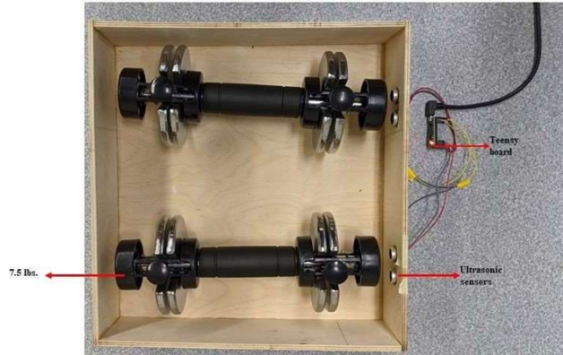
Fig. 1. Weights and Teensy board layout.
